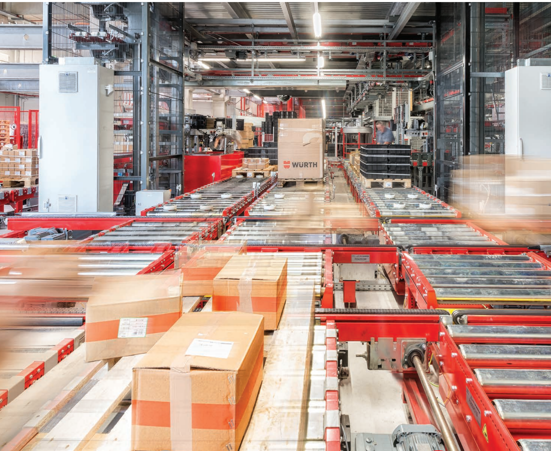
Ultra-modern technology: OSR (order storage and retrieval) shuttle warehouse
